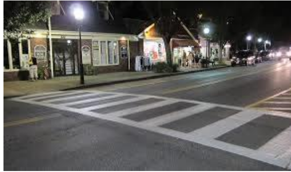
Figure 1: Laddering Type Markings
